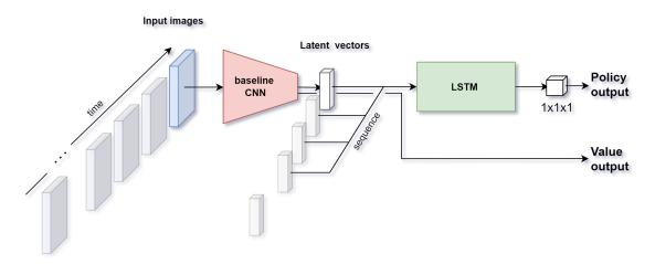
Figure 5.3: The CNN-LSTM hybrid model architecture.
