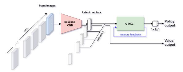
Figure 5.4: The CNN-GTrXL hybrid model architecture.
