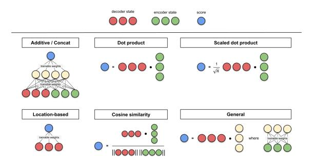
Figure 2.5: Illustrated alignment functions. (source: [17])
