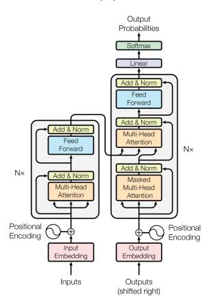
Figure 2.8: Transformer architecture. (source: [37])
