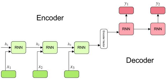
Figure 2.3: Seq2seq model architecture for general case, where input and output sequence length can be different. (source: [18])
