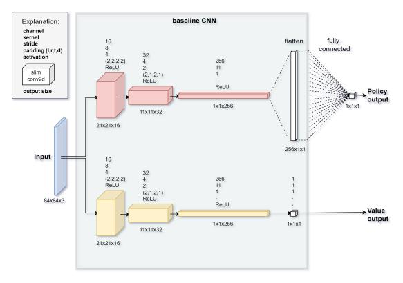
Figure 5.1: The baseline CNN model in detail.
